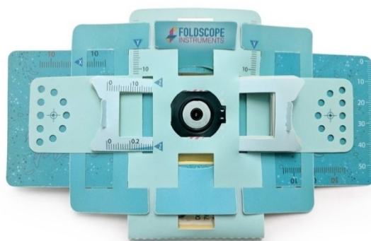
Figure 2. Foldscope - the paper microscope used for the study
